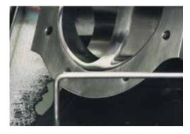
necessary to clean assembles in between manufacturing steps to ensure contamination is not an issue. This can often be a problem when leading onto heat treatment or welding operations, as surface contaminants are easily absorbed into the upper surface layers and extremely difficult to remove.
